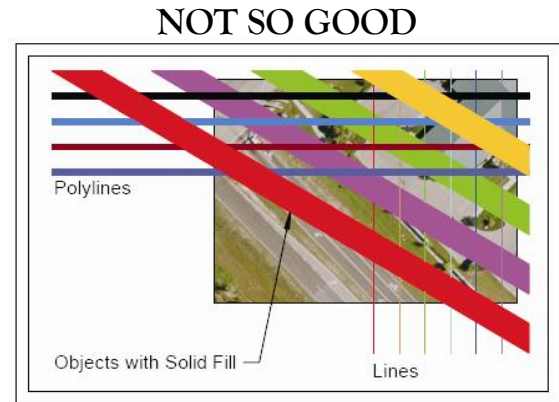
Figure 2. The “lines merge” function is not supported; overlapping CAD entities are not transparent when converted to PDF. This PDF will NOT view and print as intended.
